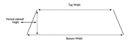
Bottom Width — Top Width < 0.50 Vertical Sidewall Height
