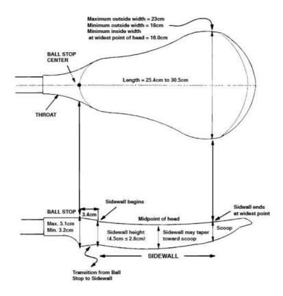
Diagram 14 Plastic/Molded Head Specification
