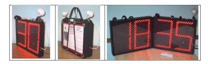
Most of the portables in use are of this type although the style of horn can vary. They are typically provided with a white hard-sided carrying case which has room for the 2 clocks, horns, power supplies, extension cords and remote.
